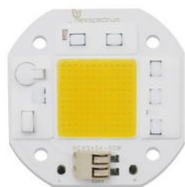
Flip chip led solution
