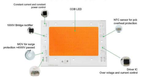
Anti-interference device multiple anti surge protection
